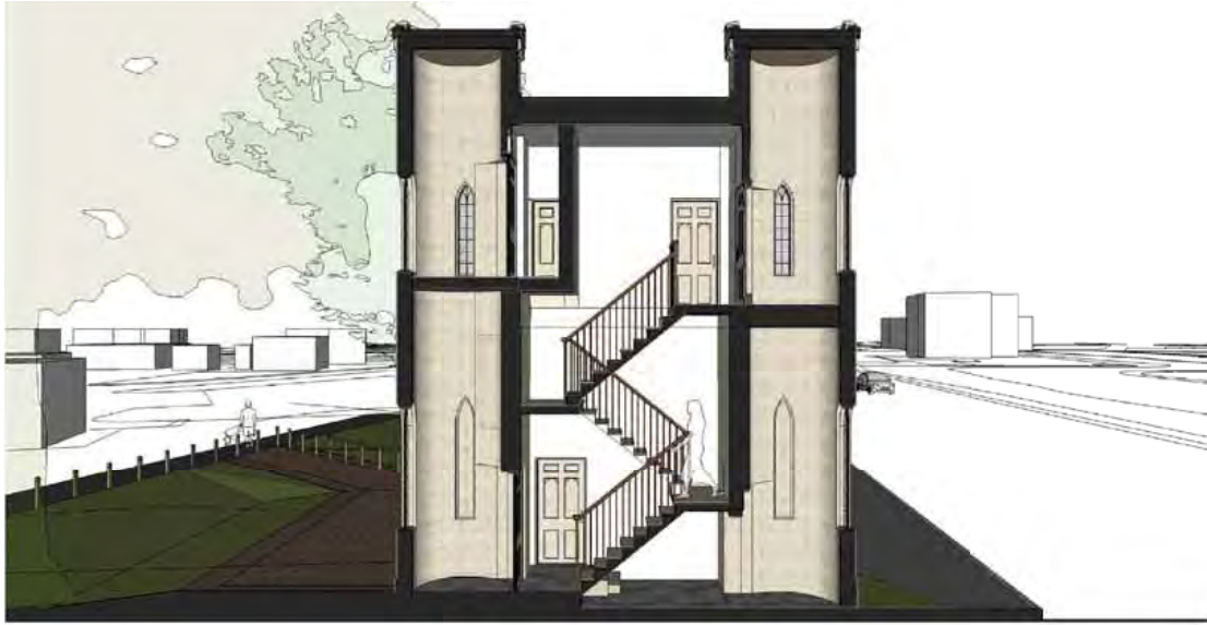
Cross Section facing East through main stair
