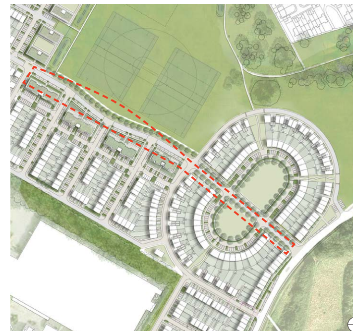
04b proposed illustrative masterplan - increase size of Hengrove Park by adjusting profile of east-west road
