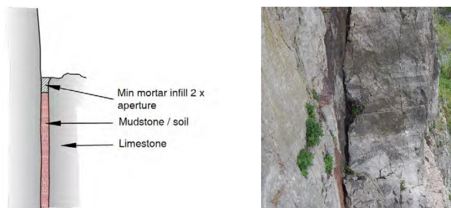
Figure 3 - Example joint dentition showing sketch cross section of dentition (left) and example of open section of JS1 joint
