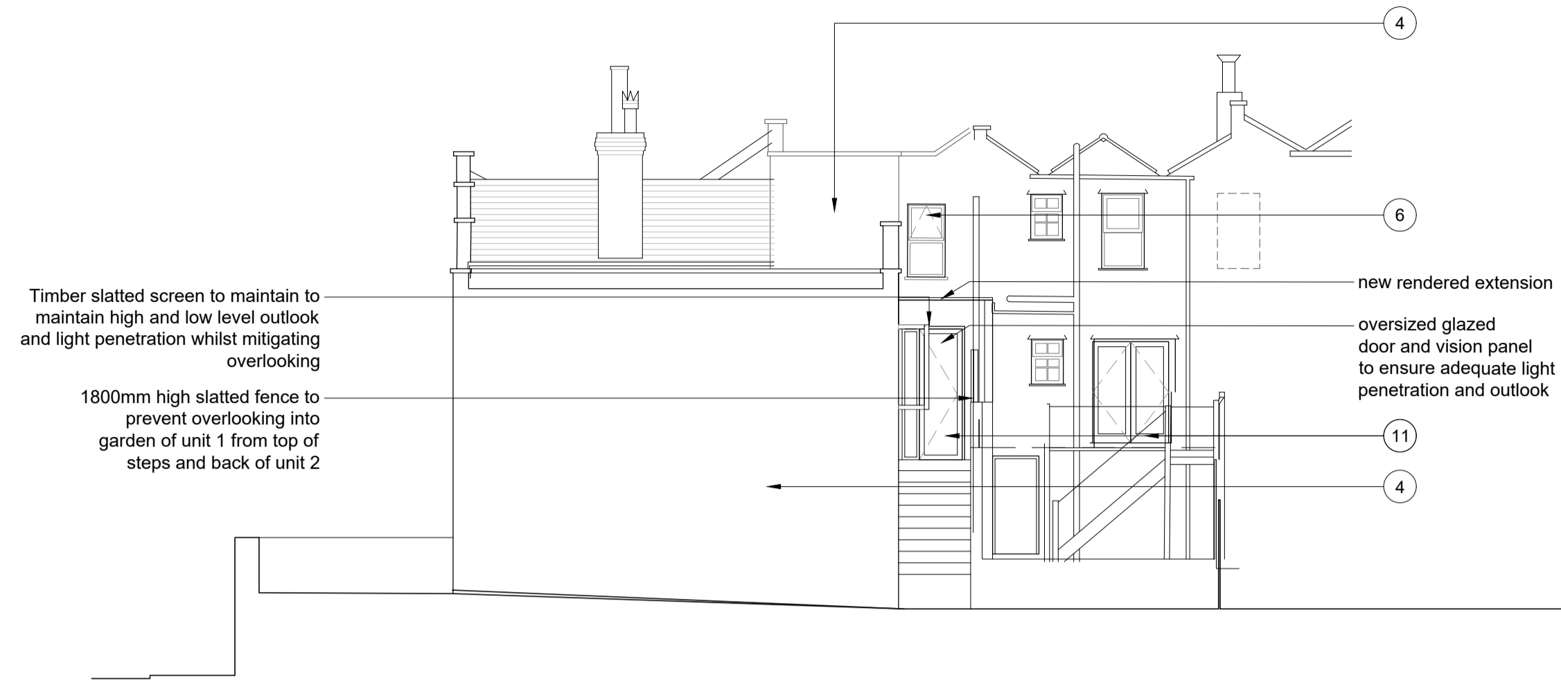
North West Elevation
